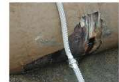
A damaged pipe joint after the 2000 landslide.
